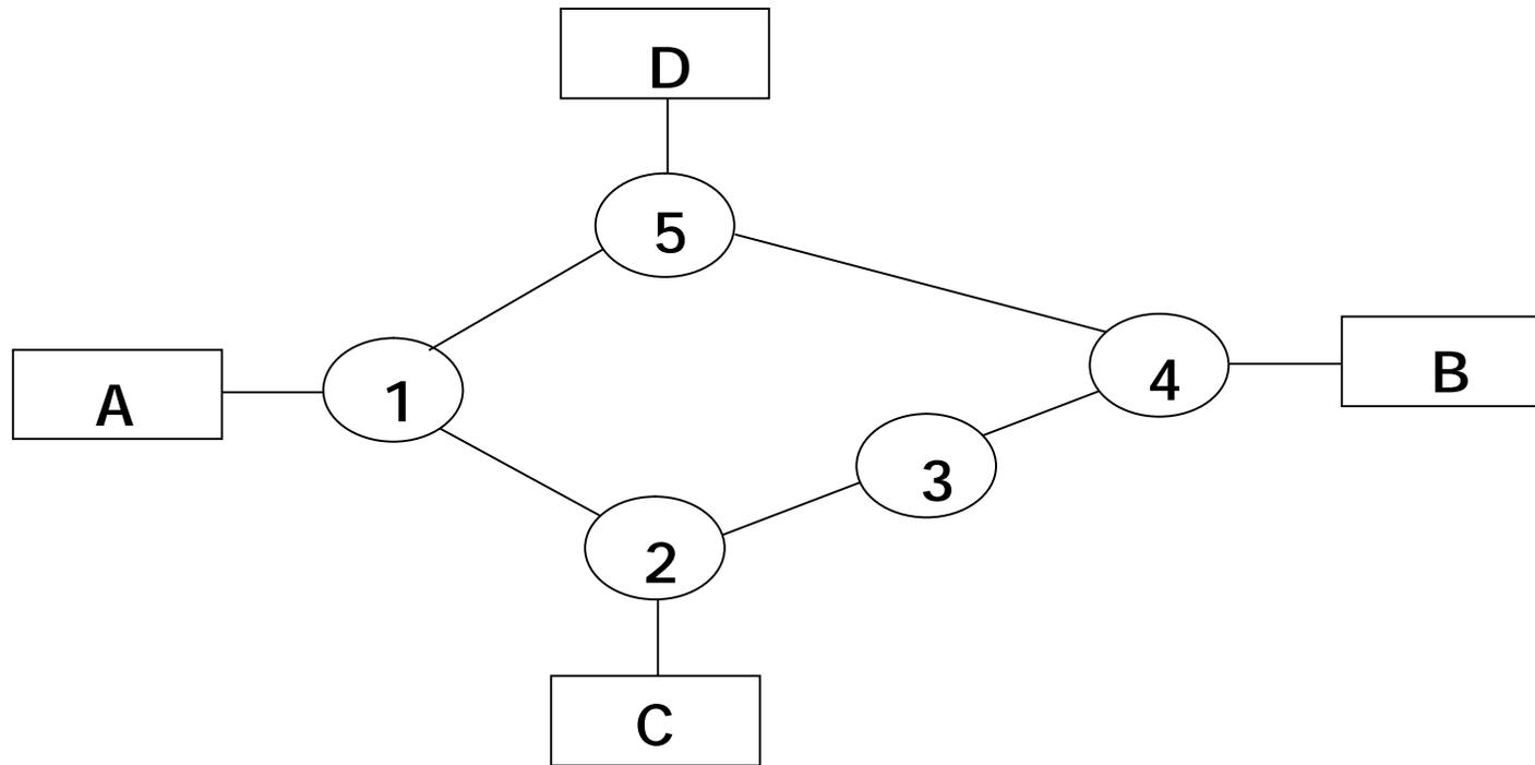
Either path 1-2-3-4 or 1-5-4 may be used to transmit a message from A to B.
